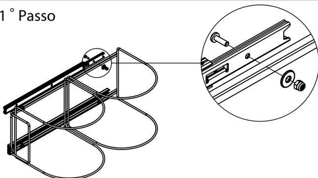
Fixe a Corrediça(C) ao Aramado(A) usando os Parafusos(F), as Arruelas(G) e as Porcas(H).
